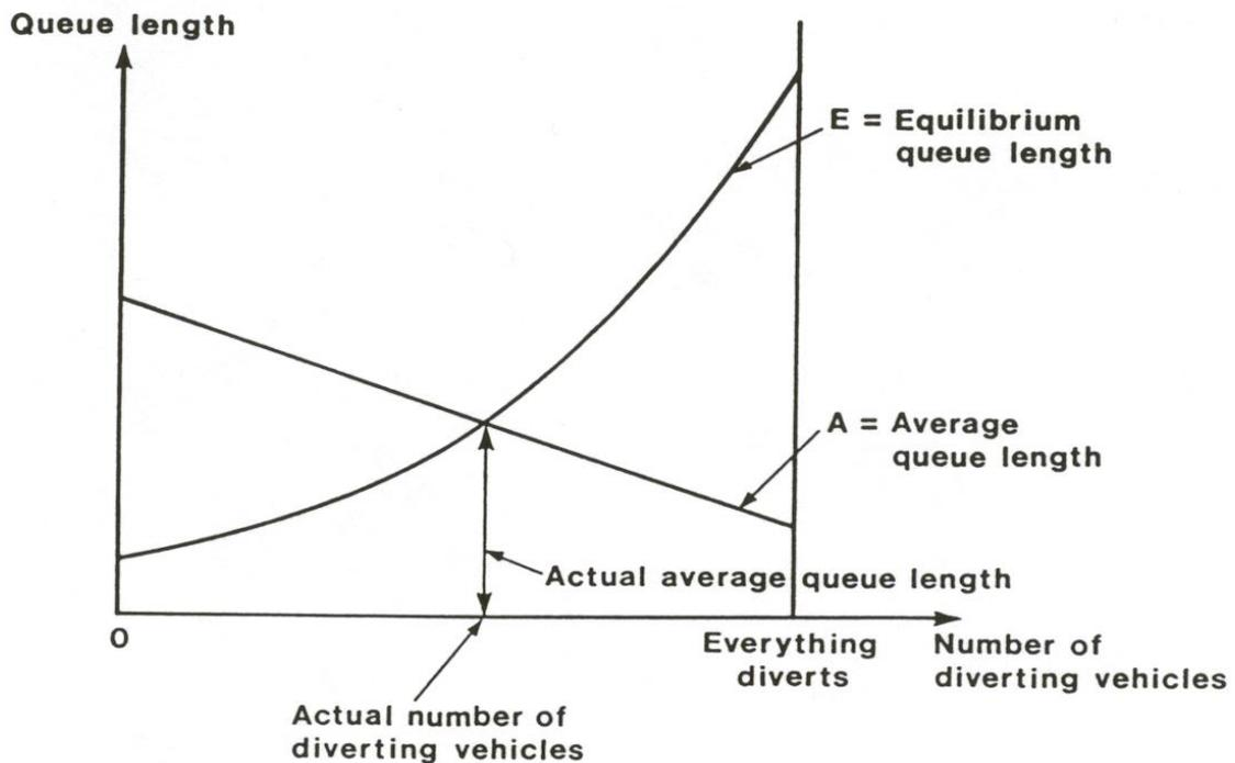
Figure 2/2: Method of Determining Queue Length and Number of Vehicles Diverting
